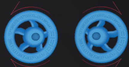
The Movement of The Turbines Reduces the Peak Brain Rotational Acceleration
